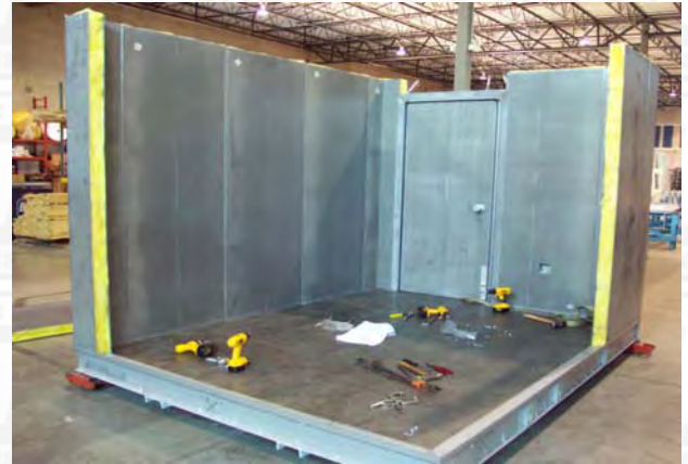
Modular Wall Panels Being Assembled Onto Base
