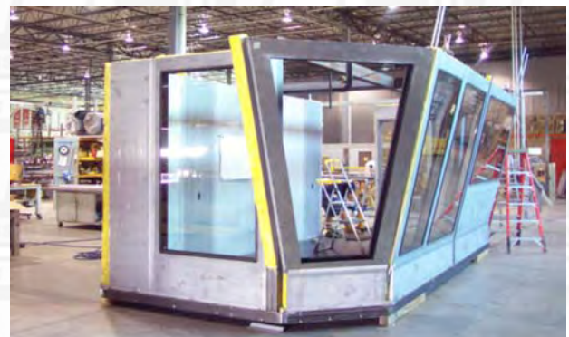
Custom Cantilevered Walls & Windows Being Assembled
