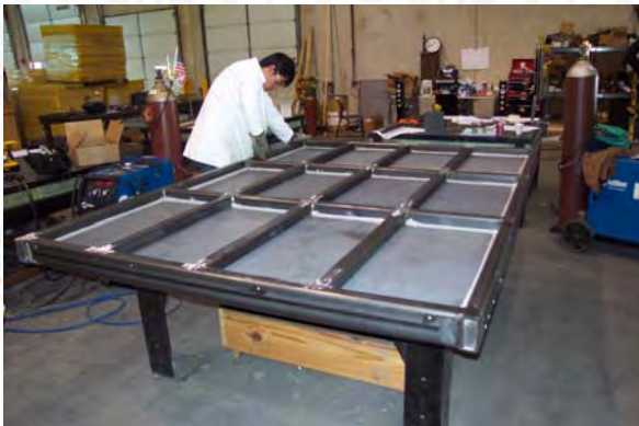
Custom Load Bearing Roof Section Being Fabricated
