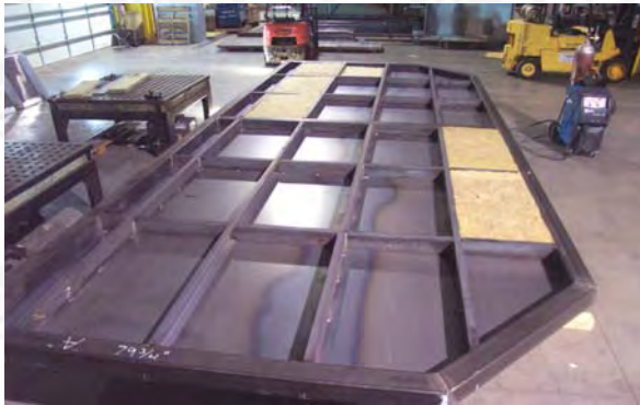
Custom Base Section Being Fabricated
